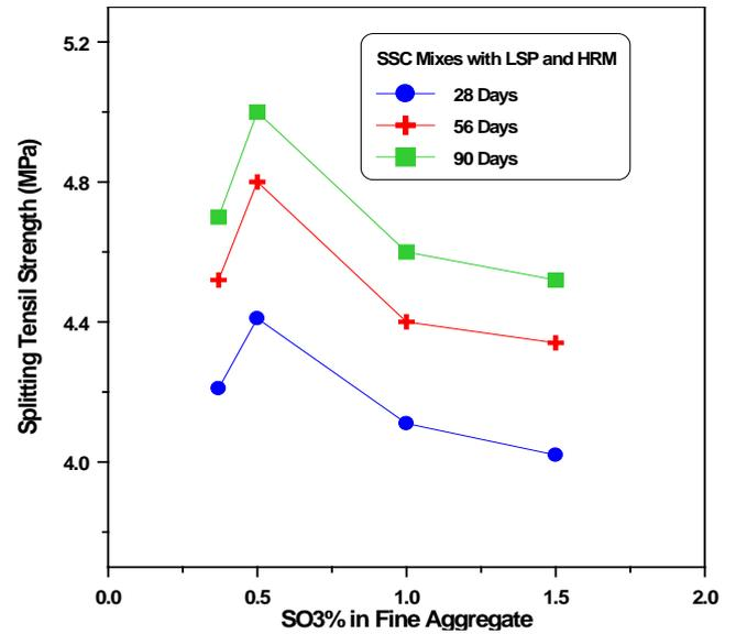
**Figure 4 :** Relationship between splitting tensile strength and SO<sub>3</sub> content in fine aggregate at different age with limestone powder filler and Metakaolin.
