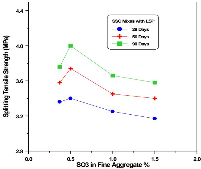
**Figure 3:** Relationship between splitting tensile strength and SO<sub>3</sub> content in fine aggregate at different age with limestone powder filler.
