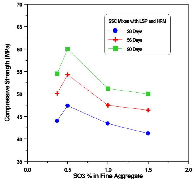
**Figure 2 :** Relationship between Compressive Strength and SO<sub>3</sub> content in fine aggregate at different age with limestone powder filler and Metakaolin.
