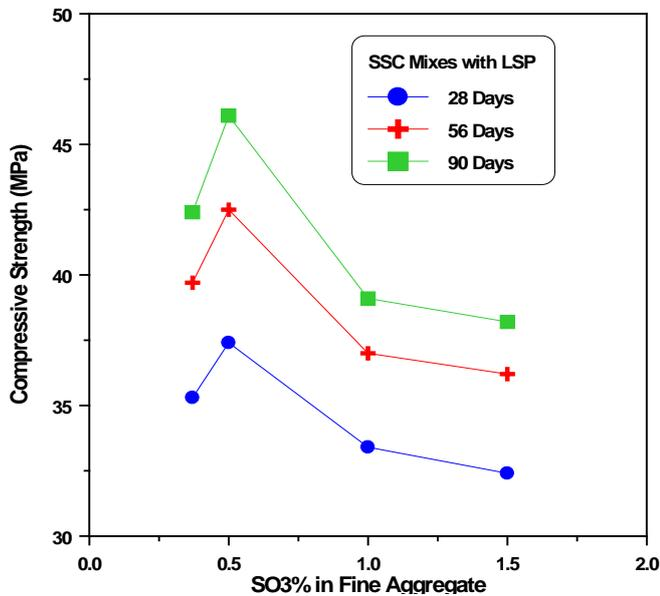
**Figure 1:** Relationship between Compressive Strength and SO<sub>3</sub> content in fine aggregate at different age with limestone powder filler.
