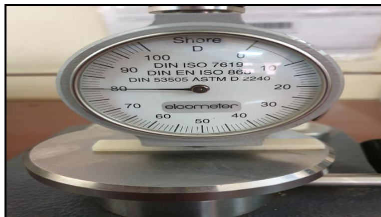
Fig. (5) hardness device (Shore-D)
