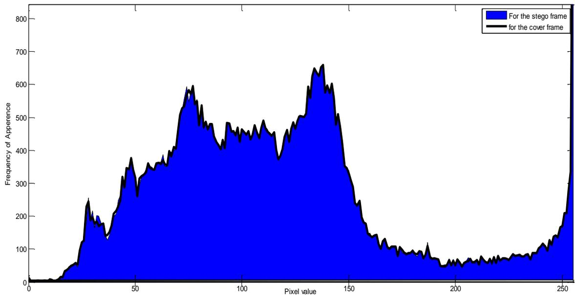
**Figure (3):** shows the histogram for the stego and cover video for frame index one.
