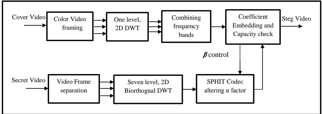
**Figure (2):** shows the proposed video steganography using SPIHT codec.
