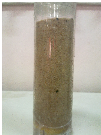
Plate (2) Sand Of Effective Diameter 0.75mm
