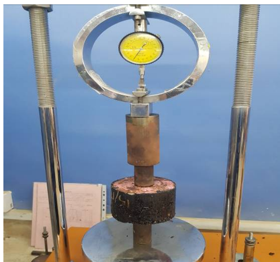
Figure 3 Double punch test device
