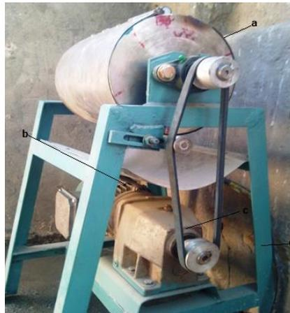
**Figure (1):** Represents the ball mill equipment that is used in the process, (a) the hexagonal drum, (b) the electrical motor, (c) the gear box, (d) is the structural frame.
