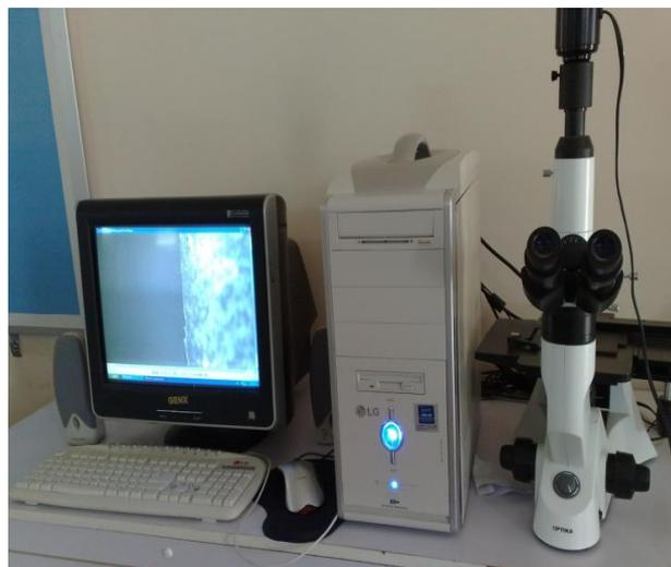
**Figure (3):** OPTIKA E Plan (40×0.65) microscope that is used in the testing.
