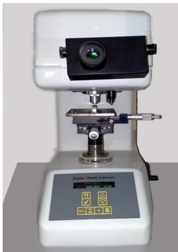
**Figure (6):** Vickers hardness tester,
