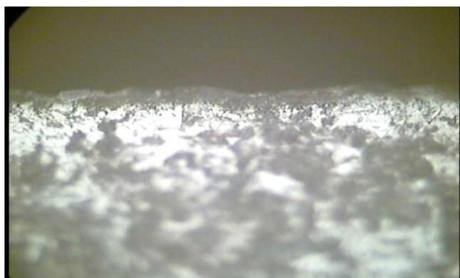
**Figure (5):** shows the hardened microstructure of (CK45), (x500).
