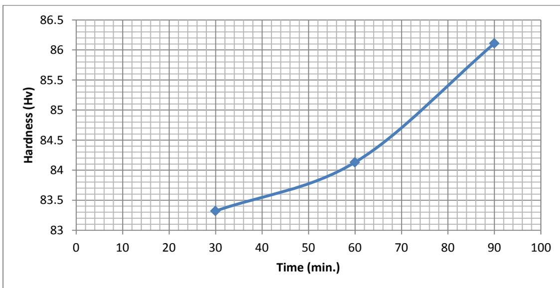
**Figure (8):** The relation between surface hardness of guide and processing time.
