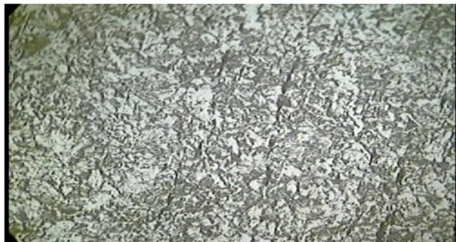
**Figure (4):** shows the non- hardened microstructure of this alloy.(400x)
