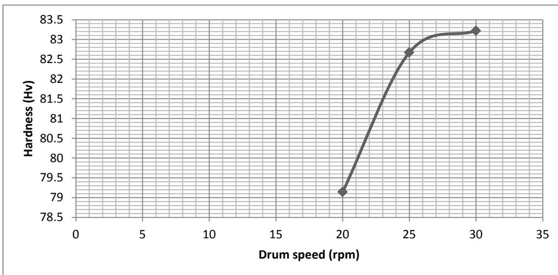
**Figure (7):** The relation between surface hardness of guide and drum speed.
