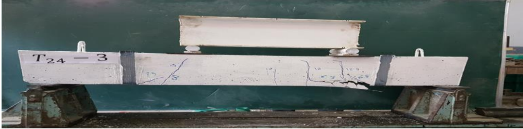
e) Beam strengthened by three strips
