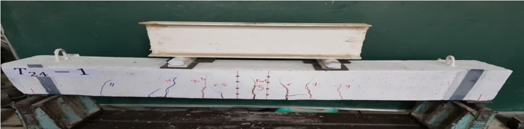
b) Beam strengthened by one strip
