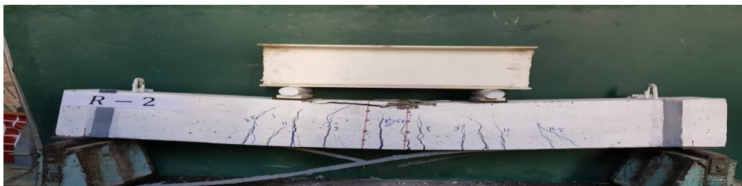
c) Beam strengthened by two strips
