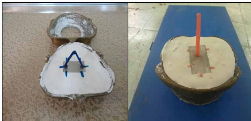
A B Figure (5): A- A major sprue attach to the middle of specimen. B- Two minor sprues attached to each other from one end and other end attached to the specimen
