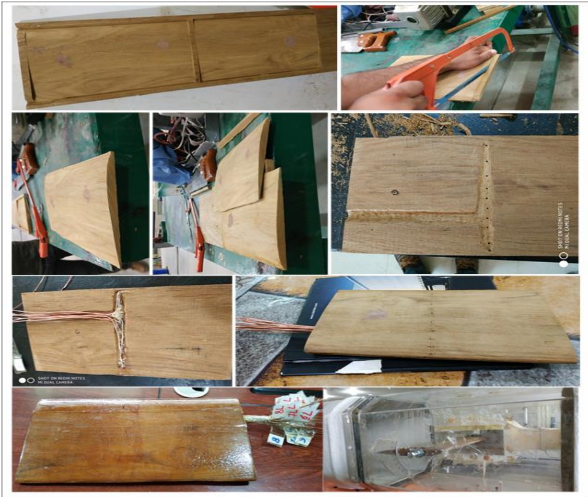
Figure (3): Steps of the Wing Manufacture and Installation it inside the Wind Tunnel.
