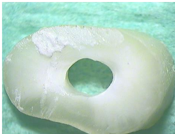
Figure (1): Inspection of the samples under a stereomicroscope at 20_ magnification and various failure modes of Biodentine samples. (A) Adhesive failure; note the clean canal wall. (B) Cohesive failure within Biodentine. (C) Mixed failure; there are remnants of Biodentine inside the canal.
