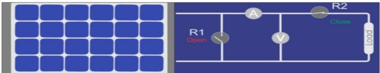
Figure 13. The electrical circuit using two relies upon R1 and R2 (one PV module)
