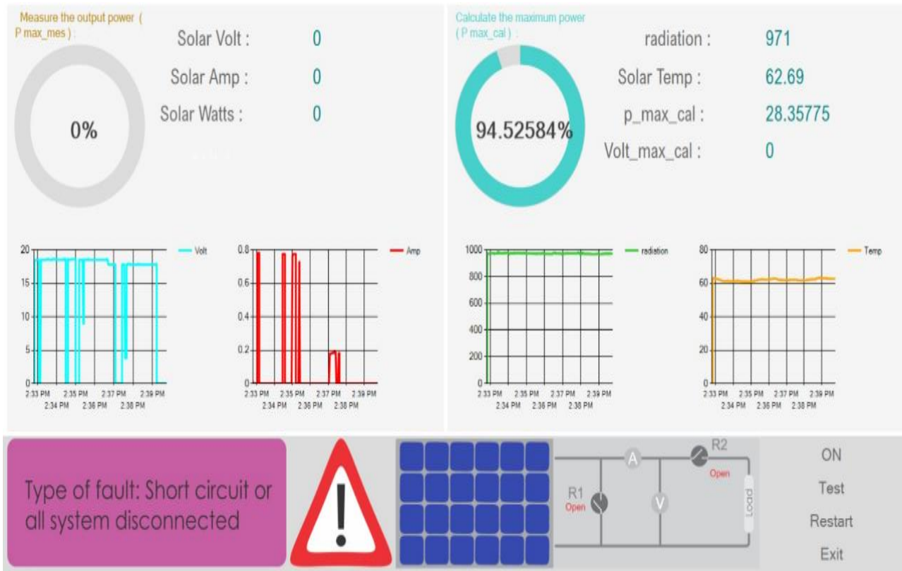
Figure 16. Short circuit or all system network disconnected
