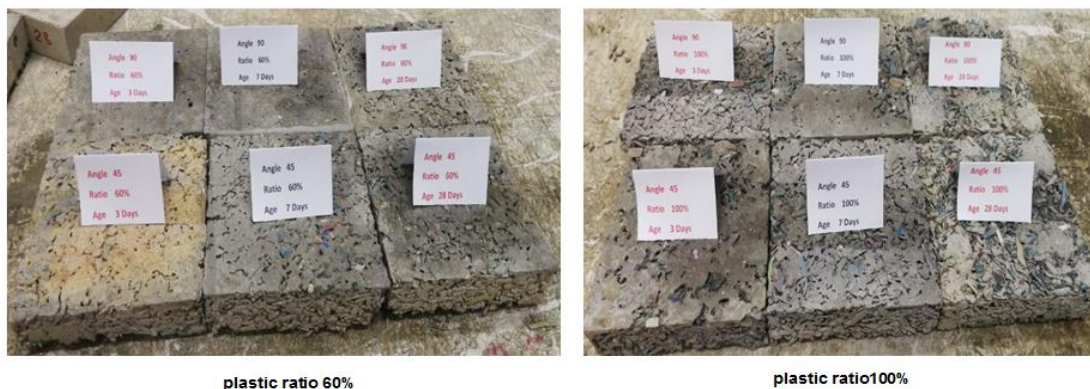
Fig 6. Depicts the effects of various inclination angles and plastic ratios on the rate of erosion at the surface of each sample under study.
