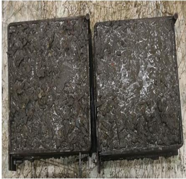
A) casting concrete samples
