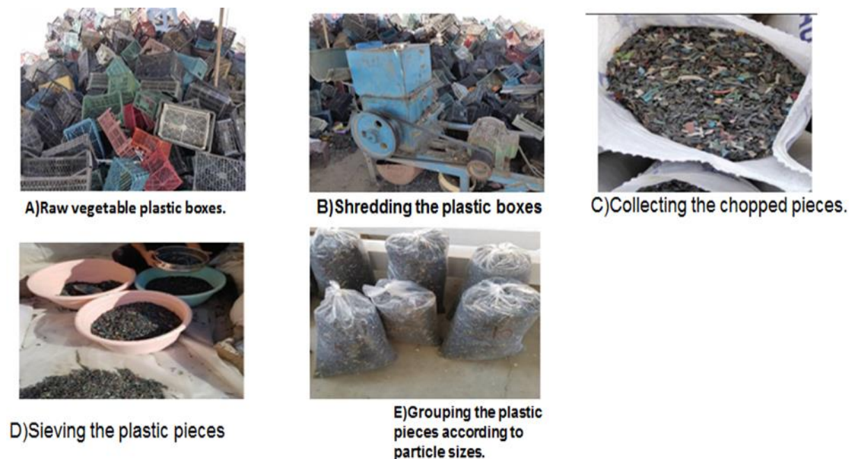
Fig 4. Depicts the process by which plastic waste is converted into a coarse aggregate. (A) Vegetable-based plastic packaging. (B) tearing up the plastic shipping containers. (C) Compiling the sliced components. Sorting the trash plastic by size (D). (E) Classifying the fragments of plastic into piles according to their particle sizes.
