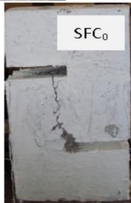
a-Specimens without reinforcement
