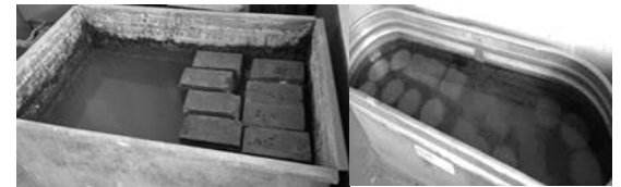
c-Push-off specimens curing
