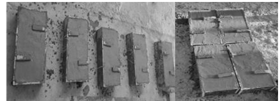
b-Casting push-off specimens
