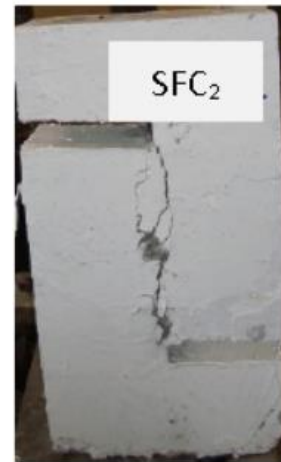
b-Specimens with reinforcement ratio (0.45%)
