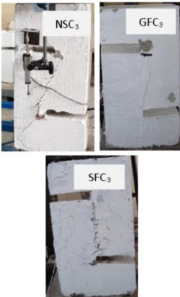
c-Specimens with reinforcement ratio (0.68%)
