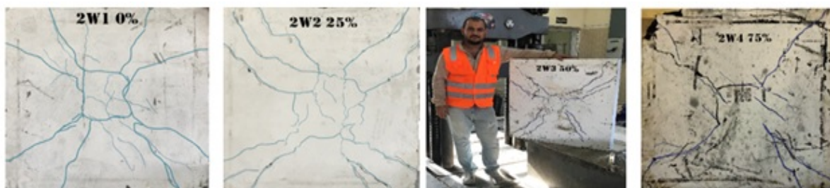
Figure 6 Cracks pattern of slabs failed in flexure.
