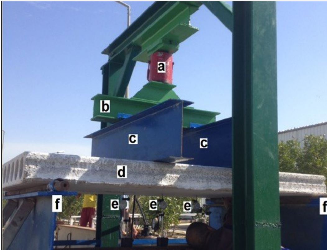
Figure 3. Specimen cross section, instrumentation and loading setup details (a) hydraulic jack. (b) spreader beam. (c) Transverse I-beams. (d) hollow core slab. (e) dial gauges . (f) support I-beams.
