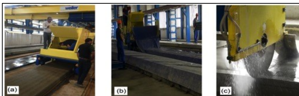
Figure. 1. (a) Extrusion process. (b) curing of the (HCS) .(c) cutting of the (HCS)
