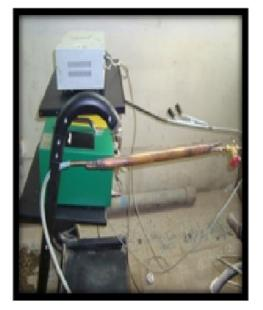
Fig. 3 EGR assembly used in present
