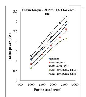
Fig. 10, Engine speed effect on BP for studied cases at HUCR and OST for
