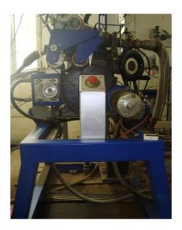
Fig.1, Single cylinder prudent spark ignition engine
