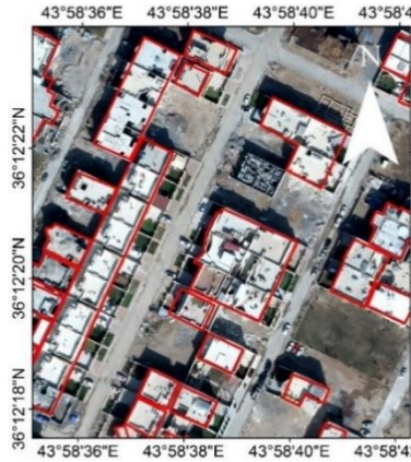
Figure 7 The red lines are the reference data ,overlain on aerial images to count the number of buildings for accuracy assessment
