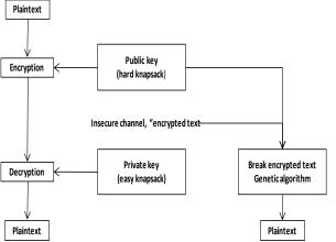
**Figure 2:** Markle-Hellman cryptosystem and cryptanalysis by means of Genetic Algorithm.
