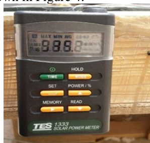
Fig.4. Digital Solar Power Meter
