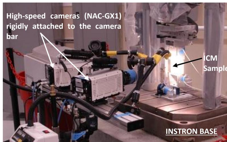
**Figure 3.** Experimental testing and Cameras set-up with lights.
