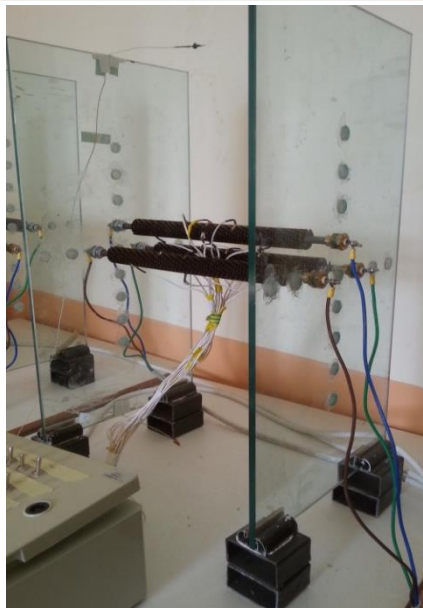
Fig. 3: Test rig for the triangle shape arrangement
