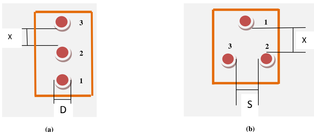
Fig. 1: (a): Three horizontal finned cylinders fixed in vertical array in line between two walls & (b): Three horizontal finned cylinders arranged in the form of a triangle fixed between two walls.
