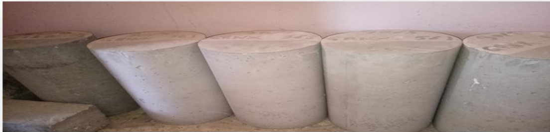
Figure 3 Demolding of test pieces
