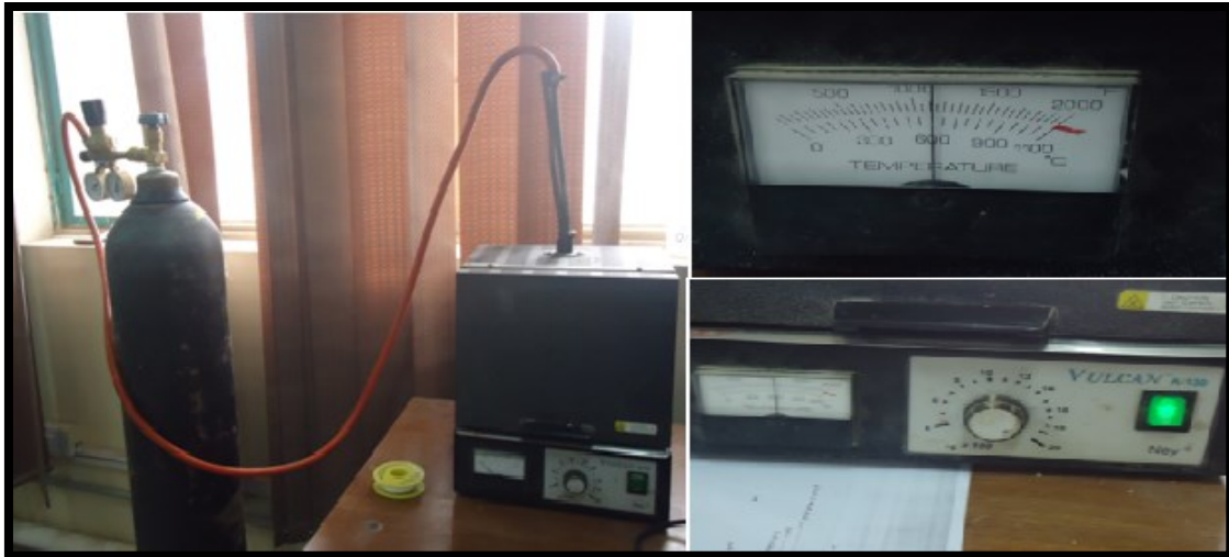
Figure 5: Sintering process (furnace and argon atmosphere).
