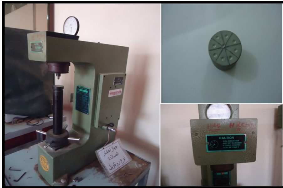
Figure 7: Rockwell hardness test device and the specimens, after hardness test.
