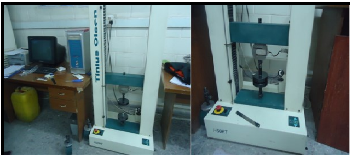
Figure 8: Universal testing machine for compression test.
