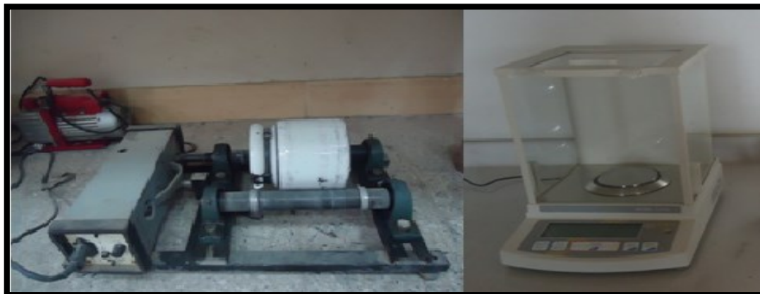
Figure 2: Blending process (sensitive electronic balance and ball mill).
