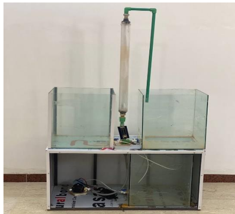
Figure 1 Photograph of the continuous (fixed bed) experimental unit.
