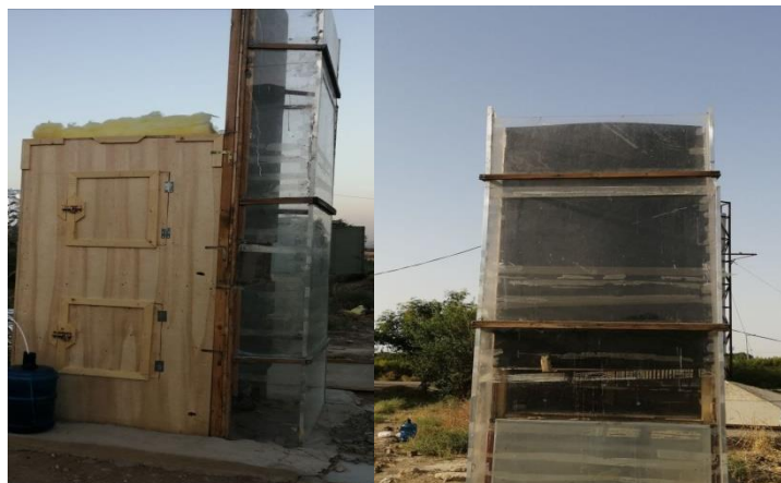
Figure 2 Two-storey building coupled with solar chimney
