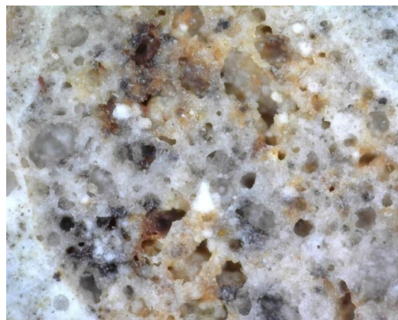
Figure 12. Optical microscopic image of microwave-sintered FAG aggregate cross-section cut (containing 8% alkali activator).
