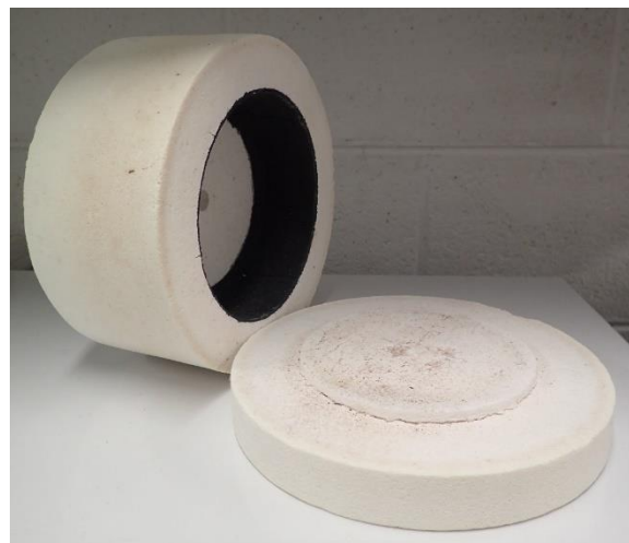
Figure 2. Image of the microwave kiln utilized in microwave hybrid heating.
