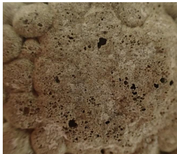
Figure 9. Image of microwave-sintered FAG aggregates containing alkali activator content of 10%.
