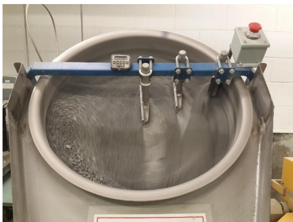
Figure 1. Image of the laboratory pelletization disc utilized in the production of green FAG lightweight aggregates.
