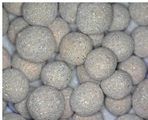
Figure 10. Image of microwave-sintered FAG aggregates containing alkali activator content of 4%.
