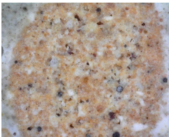
Figure 11. Optical microscopic image of microwave-sintered FAG aggregate cross-section cut (containing 4% alkali activator).
