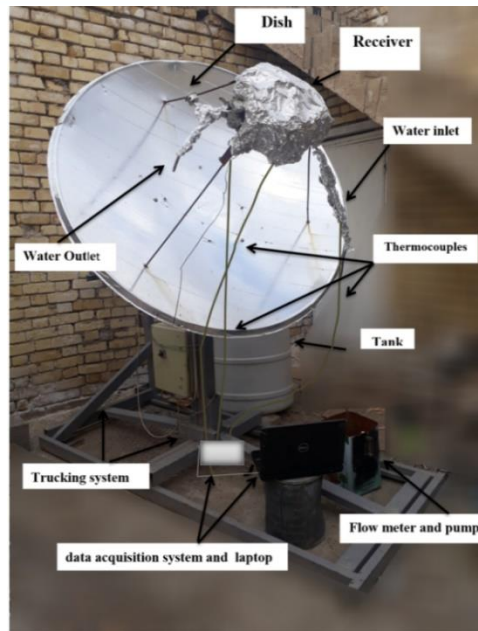
Fig.1. Parabolic Reflector of Dish Collector.
