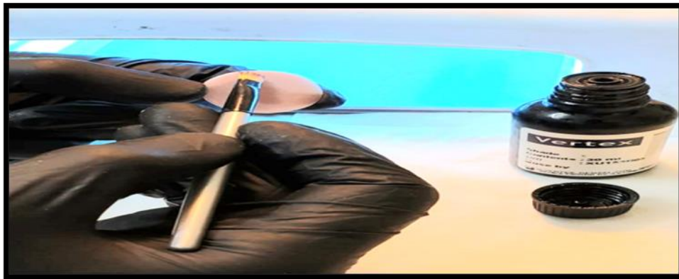
Fig. (4) : A layer of a light-cured glaze (Vertex) with a soft brush for 3 min.
