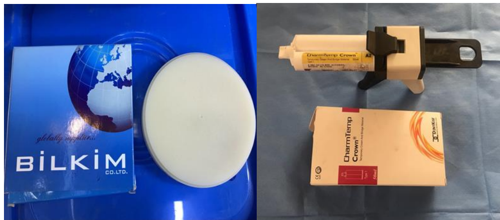
Fig. (1) (A)- dispensing gun used for mixing and dispensing of Charm temp (B)- CAD CAM flexible acetal PMMA
