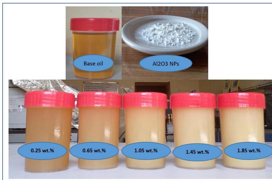
Figure 8: Testing nano-lubricants stability for 60 days at different \text{Al}_2\text{O}_3 NPs additions.
