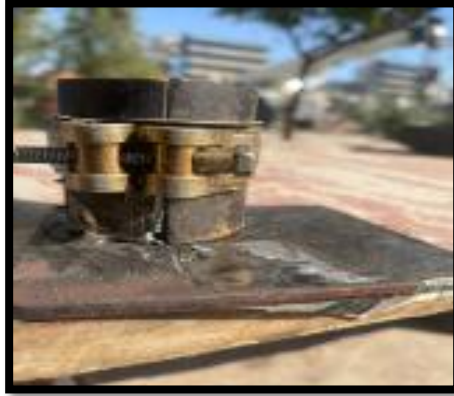
Figure 5 : The mold according ASTM C67-05
