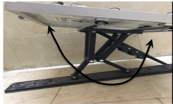
Figure 3. Free ends PV panel installed on an adjustable arm
