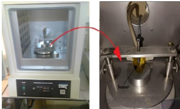
(a) Hot disc analyzer (b) Enlarged image of sensor
