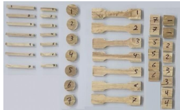
(a) Specimens used for thermal and mechanical performance tests.
