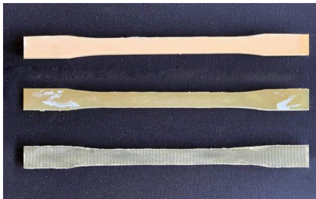
Figure 1. Tensile test samples of Epoxy/polyester and Epoxy/polyester composite with iron mesh and TiO 2 particles, respectively.
