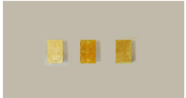
Figure 2. Compression test samples of Epoxy/polyester and Epoxy/polyester composite with iron mesh, aluminium mesh, and TiO 2 particles, respectively.
