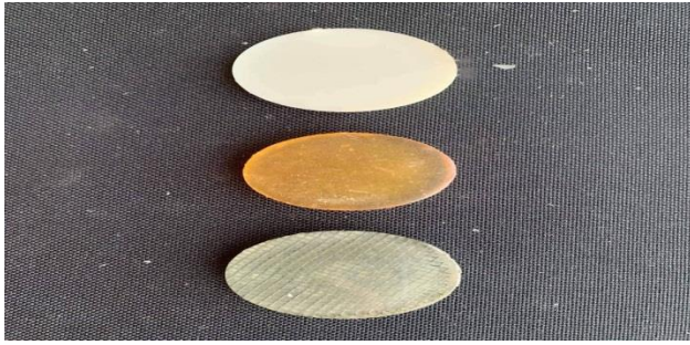
Figure 3. water absorption test samples Epoxy/polyester and Epoxy/polyester composite with iron mesh and TiO 2 particles, respectively
