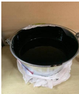
Figure 1: Crud residue from Dura refinery.
