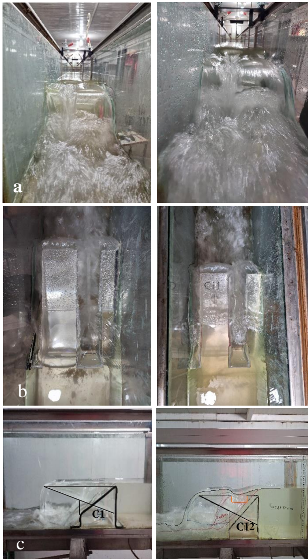
Figure 11. Flow over piano key weir a) Front view b) Top view c) Side view.
