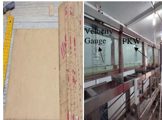
Figure 2. Material of piano key weir (left) and channel (right).
