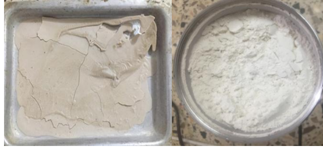
Figure 3: A. DPET after remove EG, B. Milling process of DPET.
