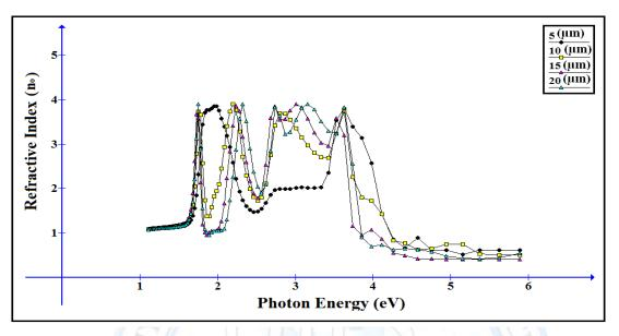
Figure. (6) Refractive index of (P V A- Green Methyl) different thickness films.
