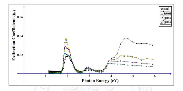
Fig. (7) Extinction coefficient of (PVA- Green Methyl) different thickness films.
