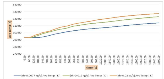
Figure 7. Variation of tank average temperature with time for three values of \dot{m}= 0.0077 , \dot{m}= 0.015 and \dot{m}= 0.02 kg/s.
