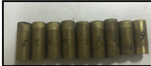
Fig.4. show brass electrode after cutting process.
