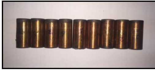
Fig.3. show copper electrode after machining process.
