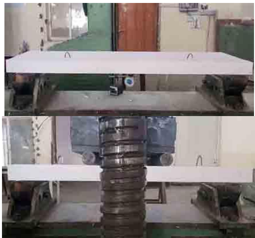
Figure 5. A slab was tested in the loading machine.
