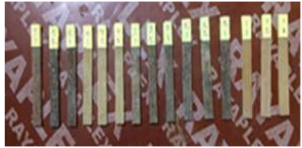
Plate (12) flexural test samples before testing
