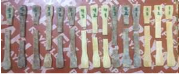
Plate (10) tensile test samples after testing
