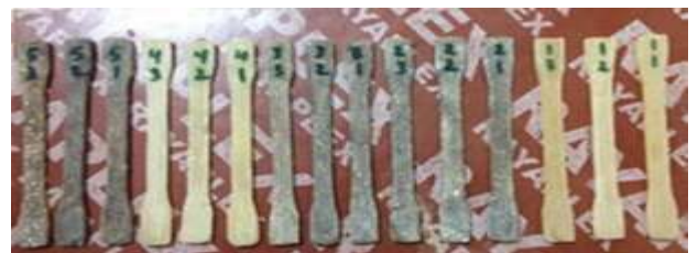
Plate (8) tensile test samples before testing
