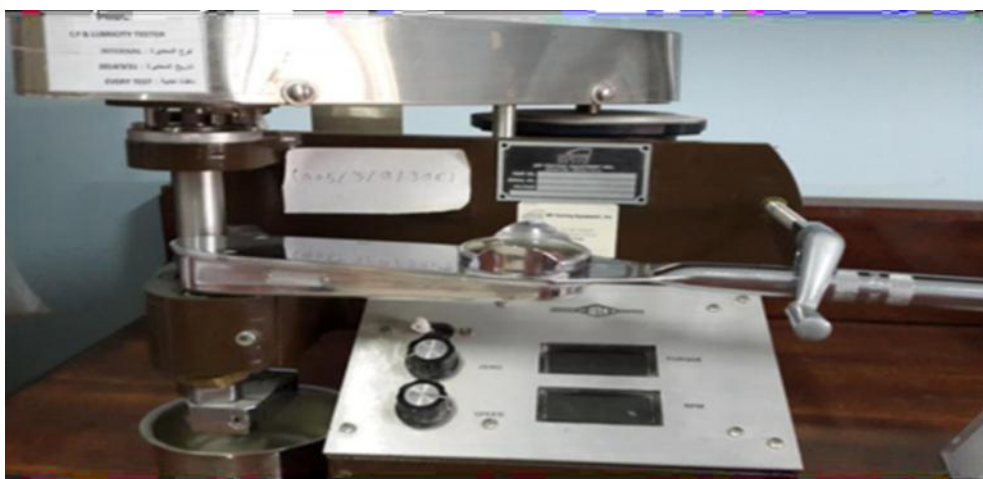
Figure 4: The device under consideration is an Extreme Pressure and Lubricity tester.
