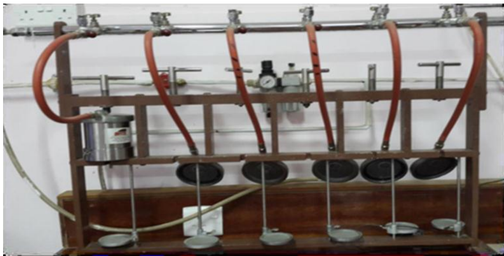
Figure 3: The device exhibits a pressure drop of 6 units due to water loss.
