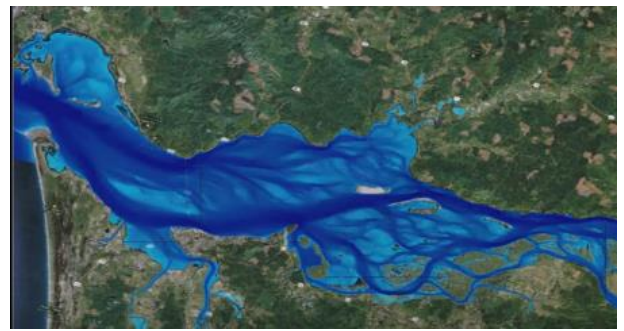
Figure 8. The spread of canal water within the agricultural lands using HEC-RAS program.
