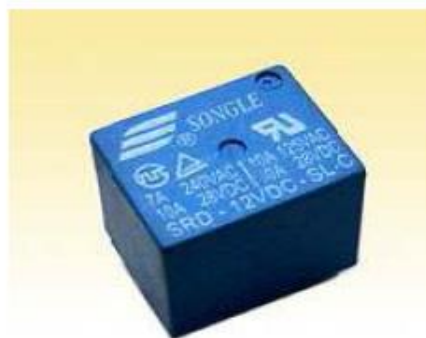
Figure 4. Relay for switching
