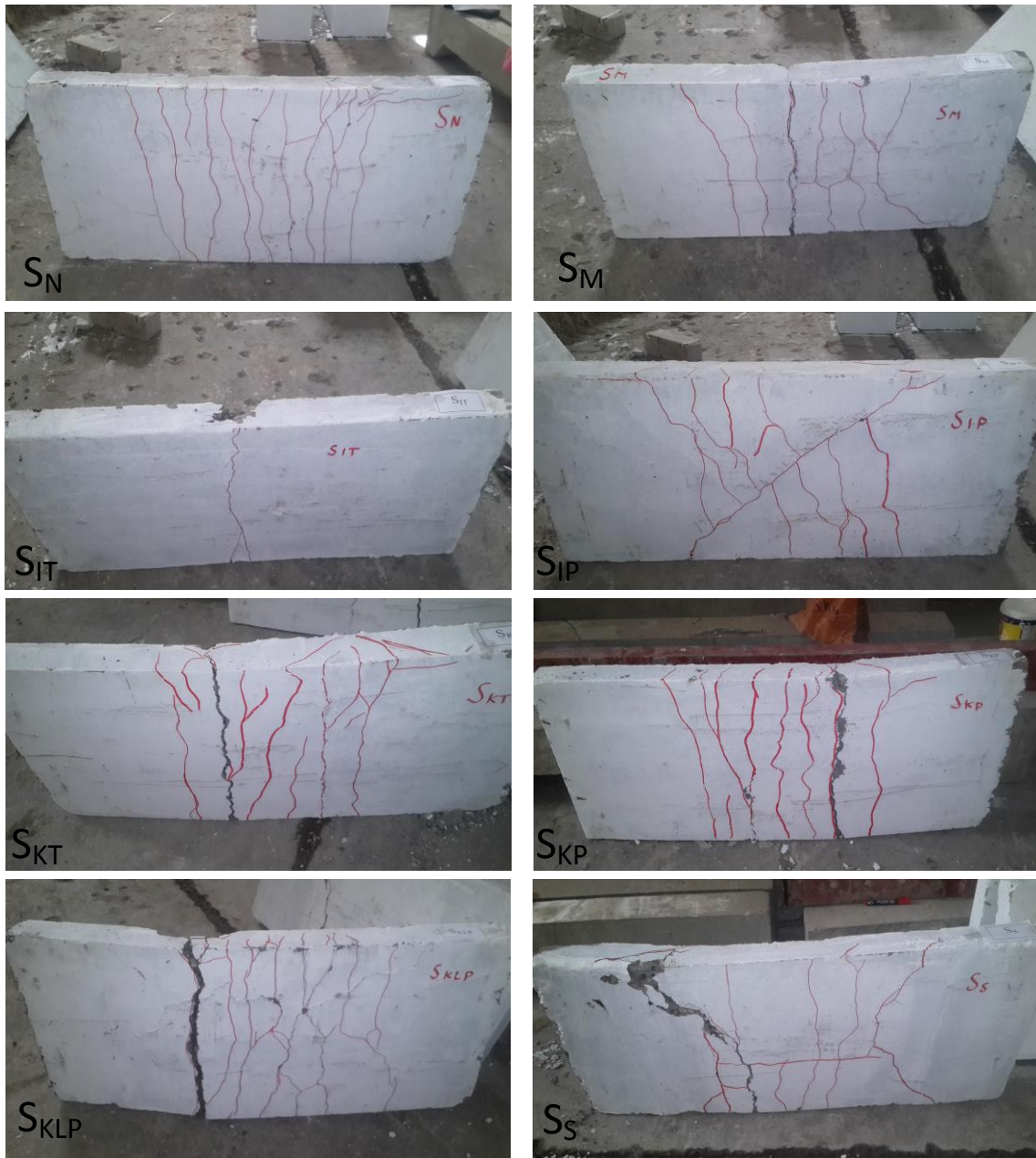
Figure (5) Pictures of crack pattern for all tested slabs
