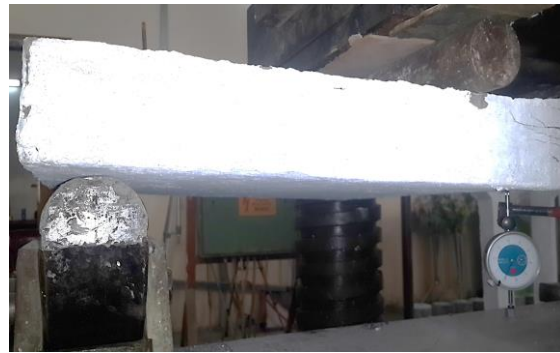
Figure (4) Dial gauge position
