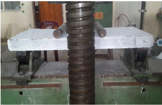
Figure (3) Slab inside testing machine
