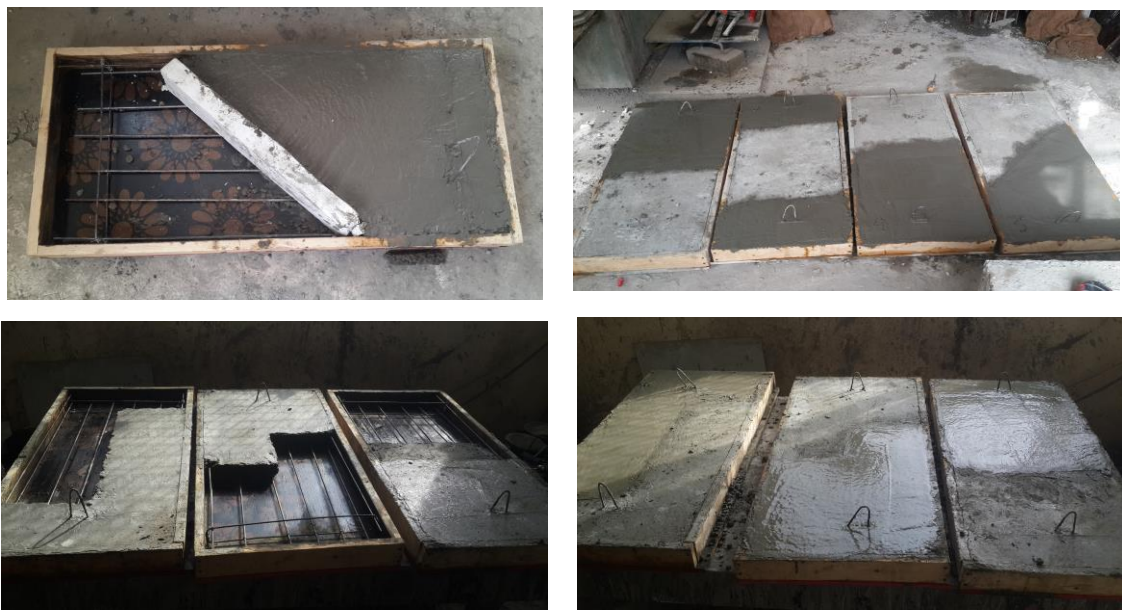
Figure (2) Casting of slabs with presence of construction joints
