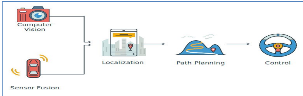
Fig.3. How computer vision works for self-driving car systems
