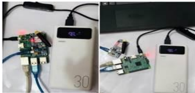
Fig. 5. Connect raspberry pi to sim868 via direct and USB
