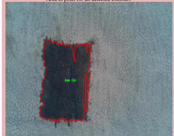
Applied the LAB algorithm and find the real area of the spill
