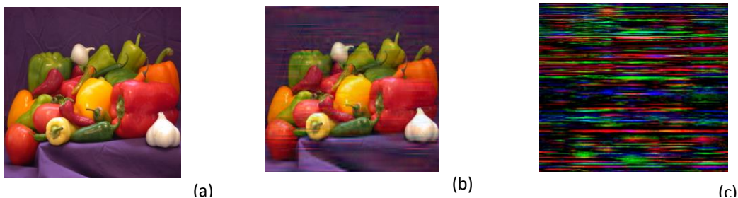
Figure.5 Key Sensitivity a) Original Image b) Decryption by correct Secret Key ( X_0 = 0.2 ) c) Decryption by Wrong Secret Key ( Y_0 = 0.20000000000001 )
